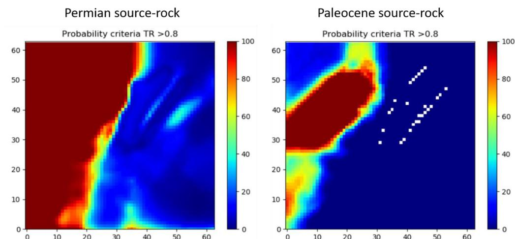
Figure 4. Map of probabilities (%) that the Permian (left) and the Paleocene (right) source-rocks reached a transformation ratio higher than 80%. (North is upward)
