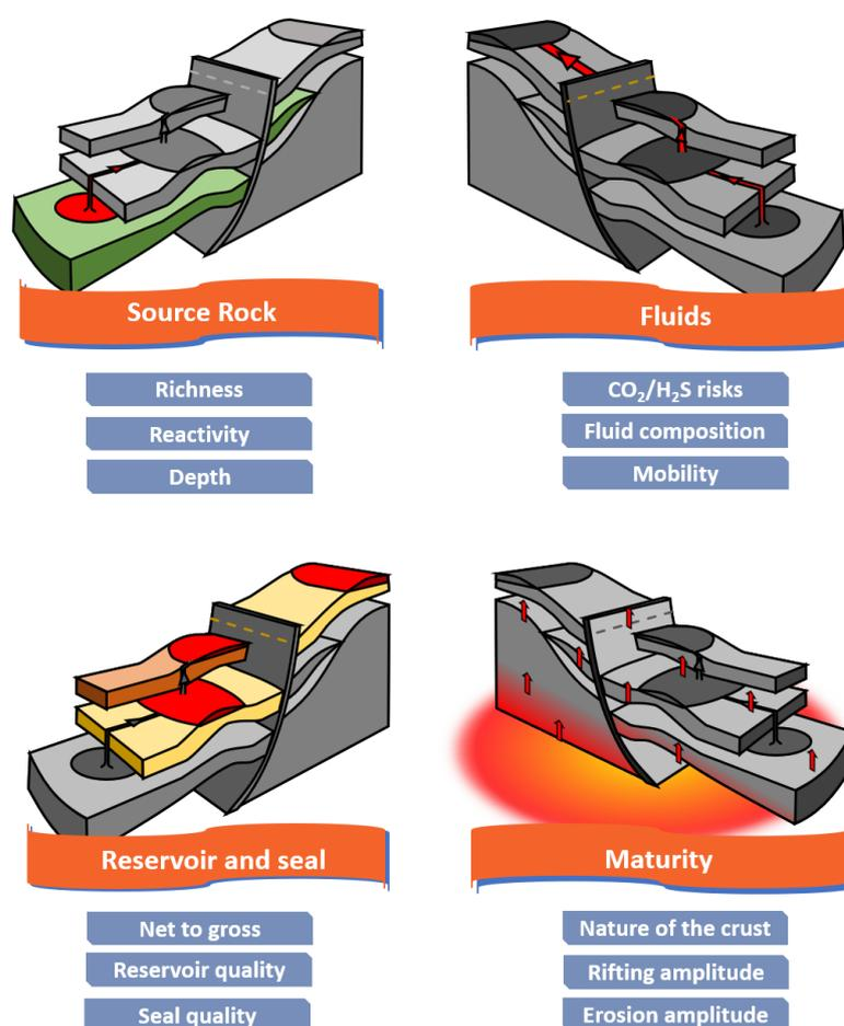
Figure 1. Description on the main elements and processes considered by the expert system for the definition of the uncertainties related to the petroleum system (modified from Hacquard, 2018).
