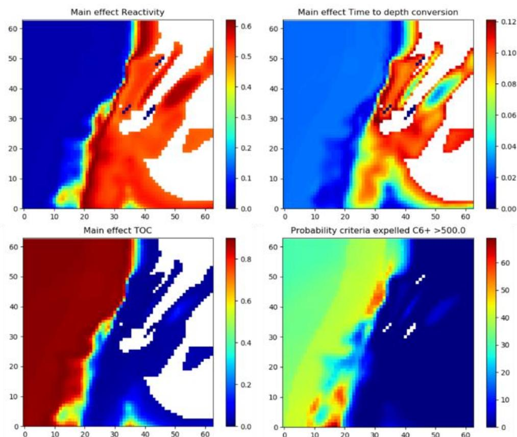
Figure 5. Maps of property contributions (%) to the variability of the expelled mass of oil from the Kimmeridgian source-rock and map of probabilities (%) that the expulsion of oil from the same source-rock is higher than 500kg/m<sup>2</sup> (bottom-right). The most prospective zones lie along the margin (bottom-right) which correspond to areas where the source-rock reactivity has a strong contribution to the uncertainty (top-left).
