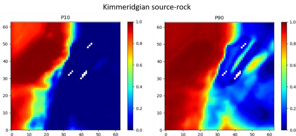
Figure 3. Percentiles of transformation ratio (%) reached by the Kimmeridgian source rock of the Levant Basin according to the defined uncertainties on source-rocks properties. (North is upward)
